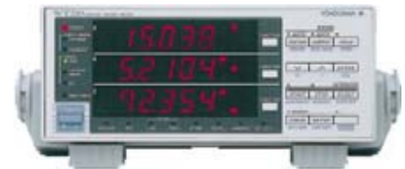
Power meter with data logging and 0.1% accuracy
